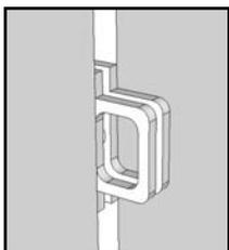
1) Install one padlock eye on the inside edge of the latch post/jamb and the other on the gate edge. The two should align
